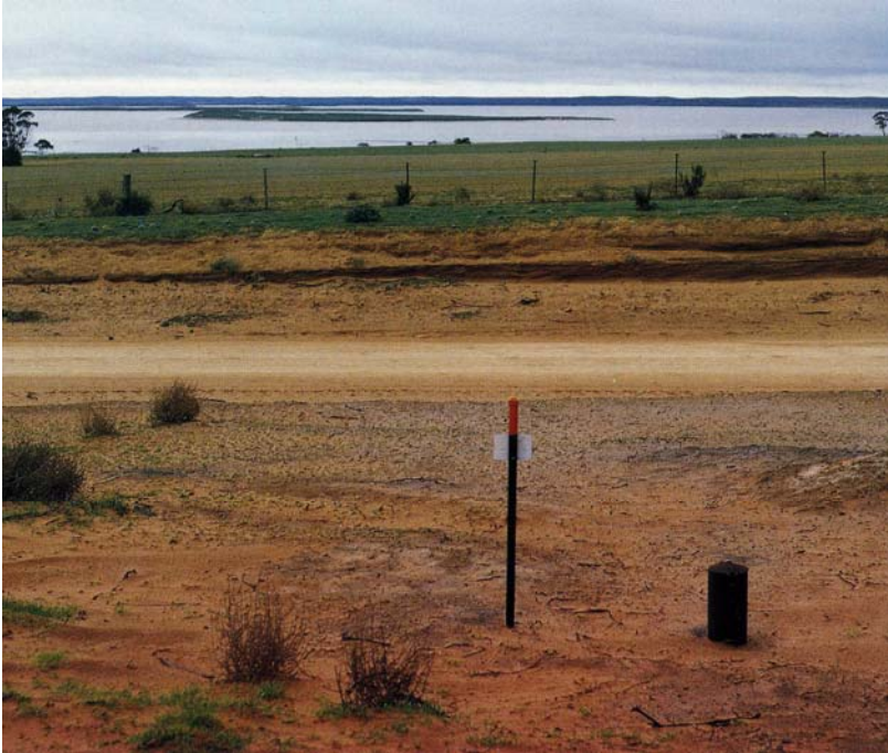
Figure 8.2 - The Bimbourie 4/5 piezometer nest, looking towards Lake Tyrrell situated about 1 km to the east. At this site, after passing through a broad transition zone, the Tyrrell reflux brines were encountered at a depth of 60 m
