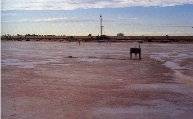
Figure 11.3 - Water level recorder situated on the lake floor at southwestern Lake Tyrrell.
