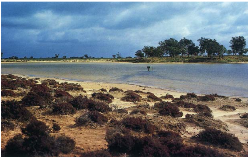
Figure 11.1 – Leopold-Stevens recorder station at Macarthur's Lake in the Raak boinka. At this site the casing is screened for 0.3 m above and below the lake floor so as to monitor either the lake level (when wet) or the water table (when dry).
