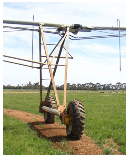
Figure 4 A well maintained, built up track – note the half-throw sprinklers on solid drops
