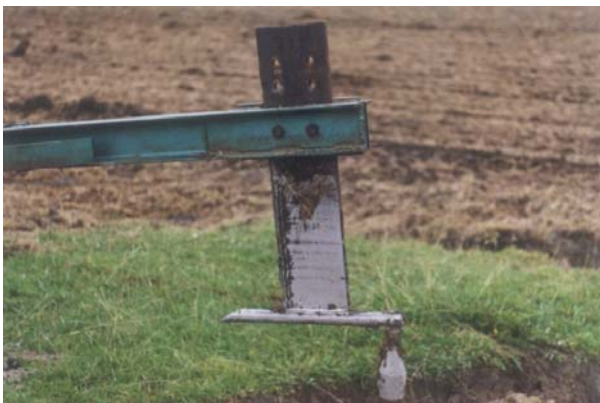
Figure 1 Mole drainer showing blade, torpedo foot and plug
