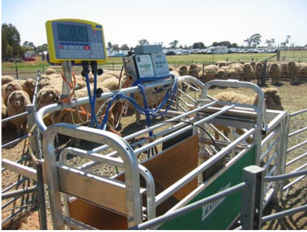
Fig 2 Panel reader set up with scale indicator and three way drafting system.
