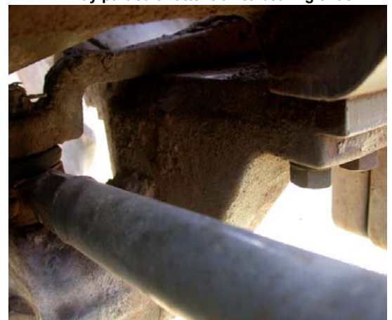
Soil built up on steering linkage
