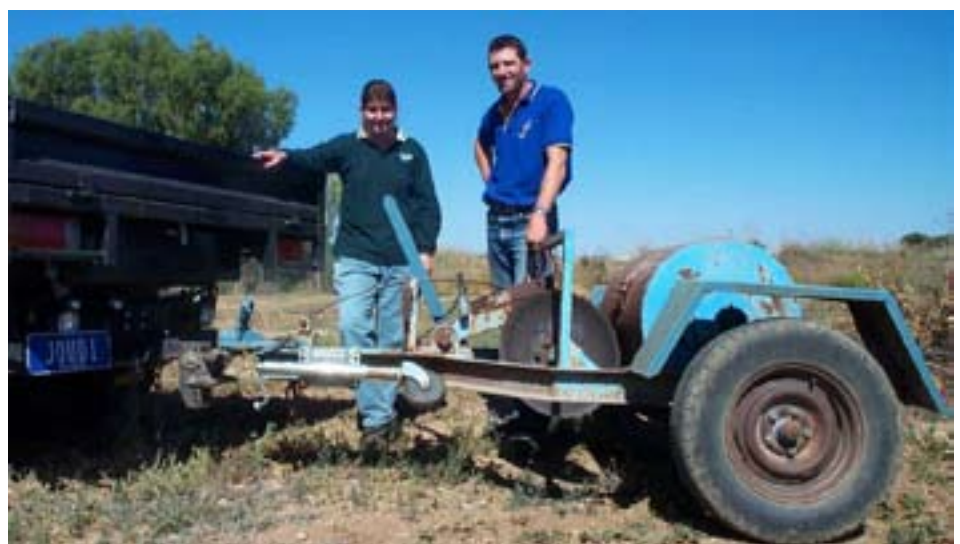
The opening on bait-laying machines needs to be closed down when changing from carrot bait to oat bait.
